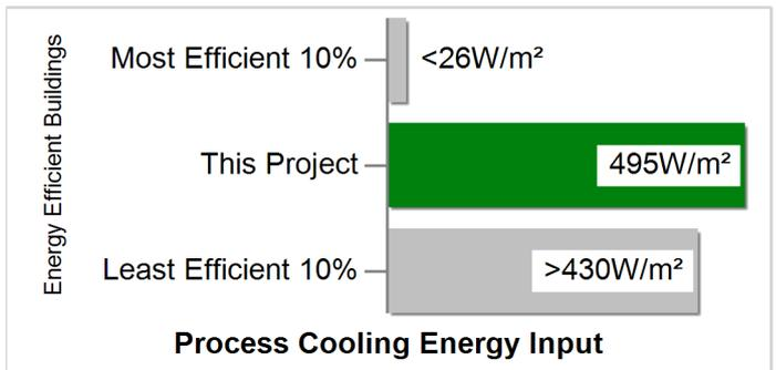
The above figures are based on the average estimated energy consumption across 4000 inspected buildings carried out using the ACE Wizard Software since 2012. The figures do not include the kW consumption from installed chilled water pumps, chilled water fan coil units, mechanical ventilation systems, remote condenser fans, cooling tower fans or system redundancy. This figure should be used as a guide only and may not reflect the accurate W/m<sup>2</sup> of the inspected facility.
