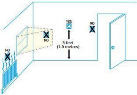
In addition to installing temperature sensors, the placement of these sensors is also of great importance as wrong placement can substantially affect the reading taken. The sensors should not be in direct sunlight, by a door or positioned above heat sources such as radiators or computer equipment. The sensors should be placed mid wall approximately 5 feet from the floor so as to provide the most accurate reading of the space temperature.
