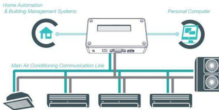
**Figure A-4 - Centralised Controller Setup for Single Manufacturer**
