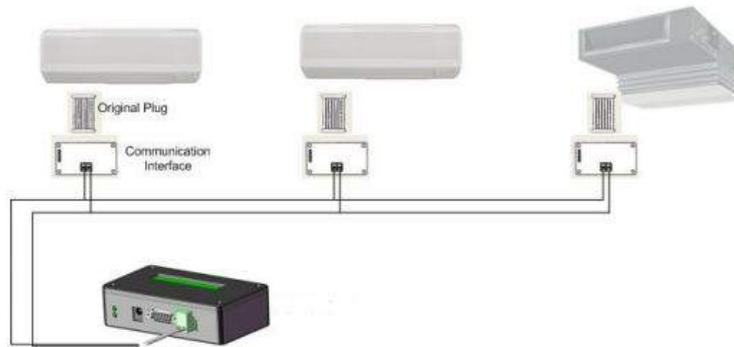
**Figure A-5 - Centralised Controller Setup for Multiple Manufacturers**
