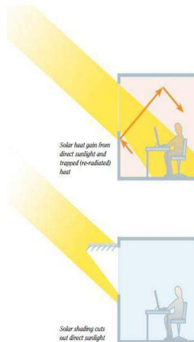
**Figure C-1 - Effects of Solar Shading**
