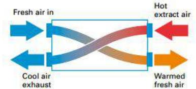
Figure I-1 - Plate Heat Exchanger
