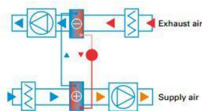
Figure I-2 - Run Around Coils
